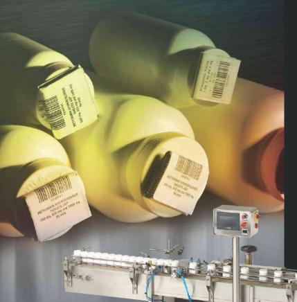
The Automatic Single Head Leaflet / Outserter Pasting Machine Model AHLI-60S, is suitable for Round, Rectangular or Square Shape Bottles with maximum speed of 50 Bottles per minute to apply Leaflet on any Side of Bottles. Specially Machine construction in completely Stainless Steel finish including machine frame structure with Stainless Steel Enclosures.
